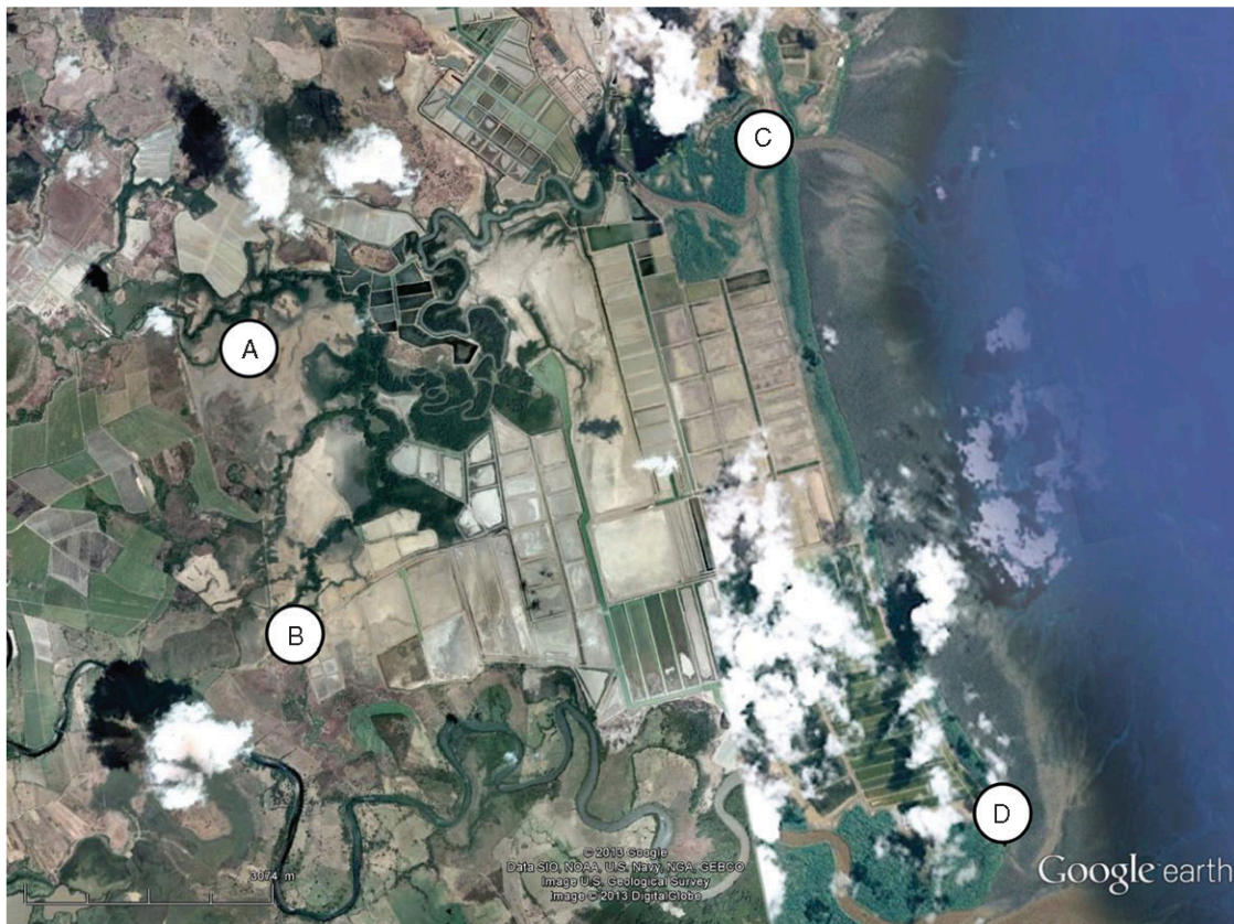
FIG. 2. The main salt works in Aguadulce, located 8°9' N, 8°31' W, 17 km south of Natá. It is protected from the sea by a 5–10 m high dam (CD). Points A and B are located 7.5 km (~2 leagues) from the sea and are only 1 m above sea level. Before the construction of the dam, the space between them and the sea was inundated by the high tide and left dry at low tide, as stated in the text. This phenomenon, not unlike what is observed in the bay of Mount St Michel (France), is rare enough to warrant that this perfect matching is not merely coincidental. In total, the salt works stretch for 32 km around Aguadulce. Source: Google Earth.
